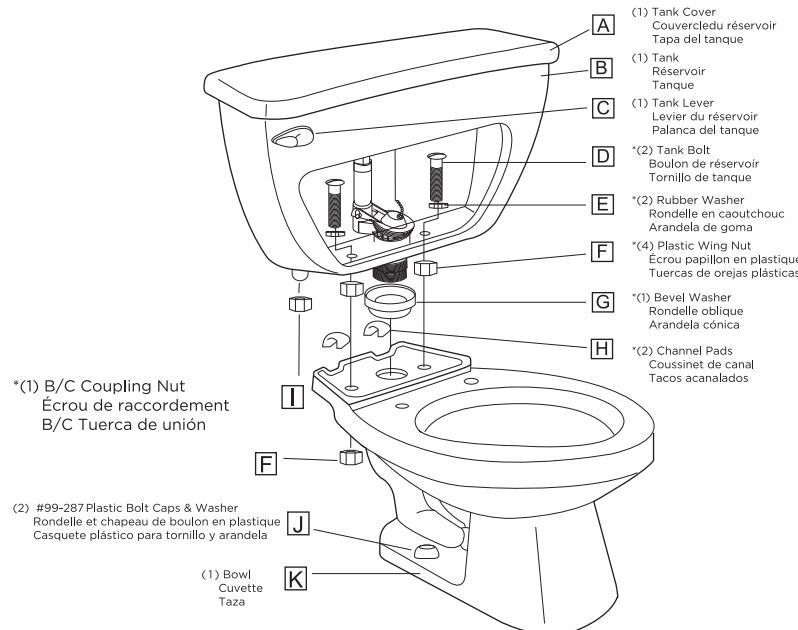
NOTE: Parts with \* are included in tank assembly kit 99-828.
