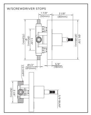
Critical Dimensions: Rough-in valve GS-323 (w/stops) & GS-327(w/stops)
