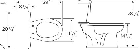
THIS FIXTURE QUALIFIES ACCORDING TO ASME TEST PROCEDURES AS A LOW CONSUMPTION WATER CLOSET WITH AN AVERAGE CONSUMPTION OF 1.6 GAL. OR LESS.
